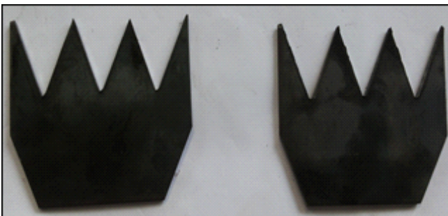
Fig.7. Blades produced after blanking & notching operation
