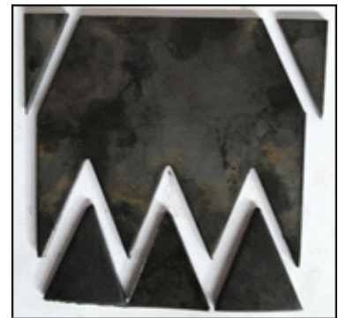
Fig.8. Improved die for blanking of blades
