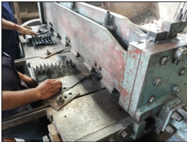
Fig.6. Notching operation for blades
